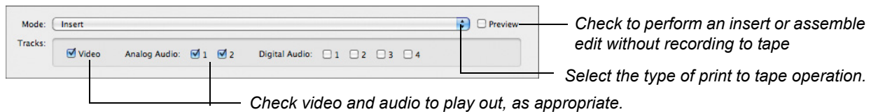
Figure 11–2. Print To Tape configuration panel.
