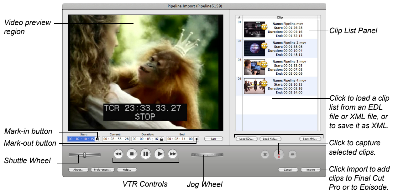
Figure 6–12. Use the Pipeline Import window to log & capture video streaming from your Pipeline.
