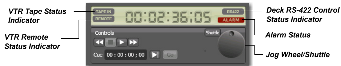
Figure 8–2. Timecode, VTR, jog wheel & control status indicators in the Log & Capture window.
