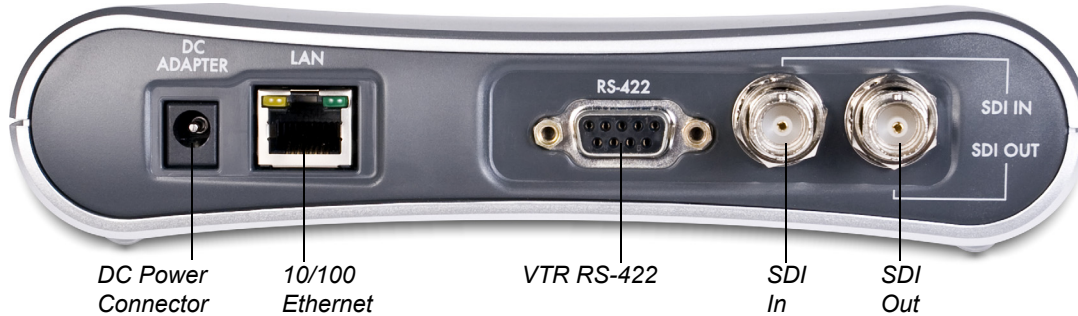
Figure 2–2. Pipeline SC rear panel
