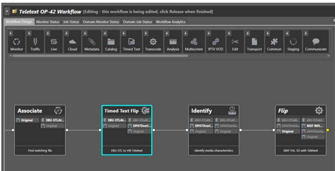
Because the VBI line graphics must be rendered onto an SD video, delivering Teletext OP-42 SD with Vantage always requires a transcode action that is specific for this purpose.
