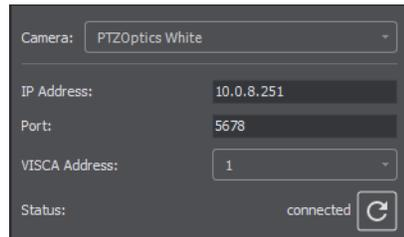
2. Select the video ingestion method from the Camera menu. This will be an HDMI or SDI capture device, or NDI if your device supports it.
