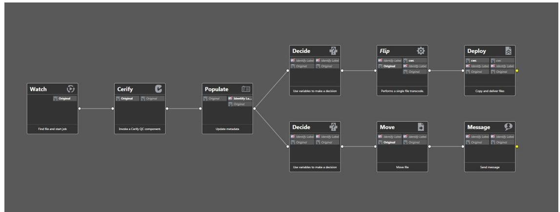
This workflow begins (as is typical) with a Watch action, configured to monitor a target location for incoming media. When the job starts, the Cerify action is executed (and the media file passed to Cerify) to perform a given QC test before transcoding the media to determine if it meets the standards or requirements you specified in the Cerify template being employed.
