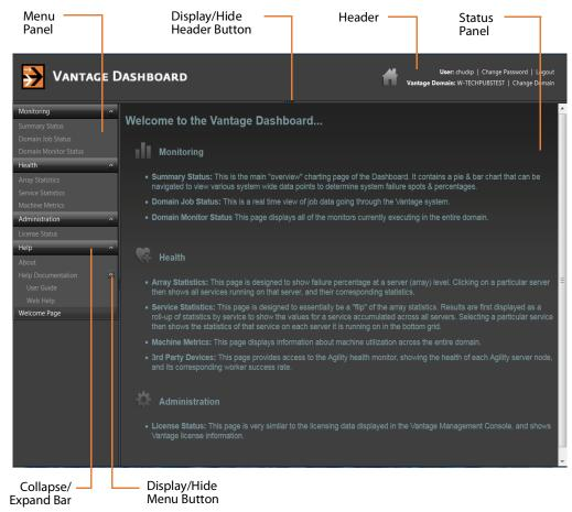
Vantage Dashboard displays information and controls in three panes: header, menu, and status. The header panel displays controls for session management, and the left menu panel displays menu selections, which are described in the Welcome page in the status panel when Vantage Dashboard starts. The status panel displays information about your domain, based on the selection you make in the menu panel.
