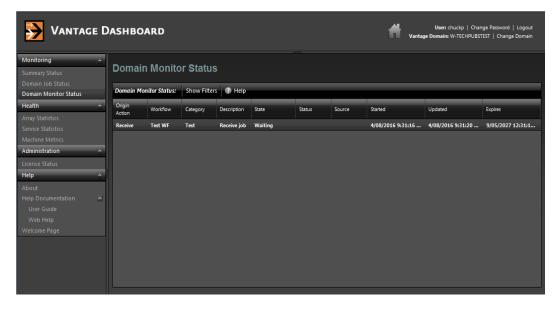
Notice that the Watch's action state is listed as *In Process*, which indicates it has started executing, and it is polling for new files. When a new file is discovered, a job is created that executes the workflow. Actions may also be *Waiting*—the state that the transaction enters while Vantage is determining which service should process it. A transaction remains in Waiting state until it is accepted by a service for processing.
