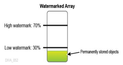
The following figure represents a watermarked disk array with permanently stored objects with a total size that is less than the Low Watermark, and temporarily stored objects with a total size that is higher than the Low Watermark:
