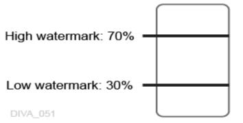
The following figure represents a watermarked disk array with permanently stored objects with a total size that is less than the Low Watermark:
