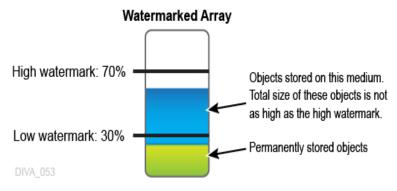
The following figure represents a watermarked disk array with permanently stored objects with a total size that is less than the Low Watermark, and temporarily stored objects with a total size that has reached the High Watermark level. In this figure the temporary objects have now reached the High Watermark, and will be removed using one of the two methods available (*Last Access Time or Largest Object Size*) until the level reaches the Low Watermark.
