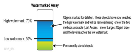
The following figure represents a watermarked disk array after the temporary objects have been deleted down to the Low Watermark. Objects have now been deleted (*either by Last Access Time or Largest Object Size*) and the Low Watermark has been reached. At this point, object deletion stops until the High Watermark is reached again; then the process repeats.
