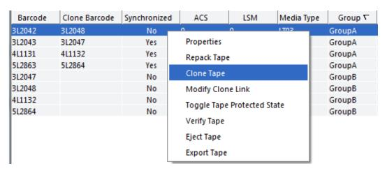
After one or more archives to a Tape Group containing a Clone Tape Group, users can manually clone the tape containing the newly archived objects. For example, upon archiving of 6 objects to a Tape Group called GroupA configured with a Clone Tape Group named GroupB, a user can clone the tape containing the newly archived objects using one of the aforementioned methods.
