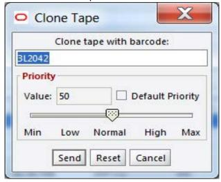
During the first clone of a Source Tape, an empty tape contained in the set associated with the Clone Tape Group is selected. The selected tape will be of the same type as the Source Tape, and equal to or greater in size. The newly selected Clone Tape is marked as protected.
