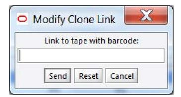
**Note:** If a user attempts to link to a compatible non-empty tape, they will be prompted with a warning to verify that they really want to link to a non-empty tape as shown in the following figure. Two tapes are compatible if they have the same format, type, total size, and last written block.
