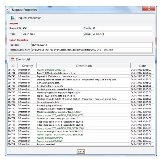
The resulting exported XML file(s) contains a new element named cloneBarcode. It is used during import to restore the clone Storage Link. It also has the lastCloneDate for the Source Tape that is also restored during import.
