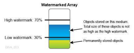
The following figure represents a watermarked disk array with permanently stored objects with a total size that is less than the Low Watermark, and temporarily stored objects with a total size that has reached the High Watermark level. In this figure the temporary objects have now reached the High Watermark, and will be removed using one of the two methods available (Last Access Time or Largest Object Size) until the level reaches the Low Watermark.
