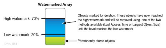
The following figure represents a watermarked disk array after the temporary objects have been deleted down to the Low Watermark. Objects have now been deleted (either by Last Access Time or Largest Object Size) and the Low Watermark has been reached. At this point, object deletion stops until the High Watermark is reached again; then the process repeats.
