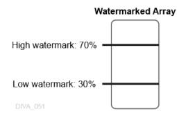
The following figure represents a watermarked disk array with permanently stored objects with a total size that is less than the Low Watermark:
