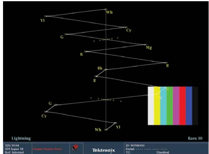
Figure 39. Lightning display with Color Bars signal.
