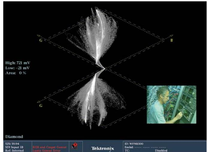
Figure 20. Live signal with green balance error.
