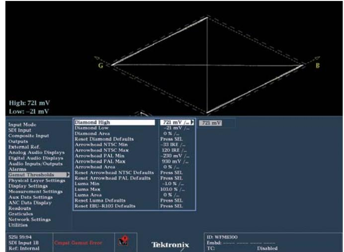
Figure 15. Configuring gamut limits on the WFM8300.
