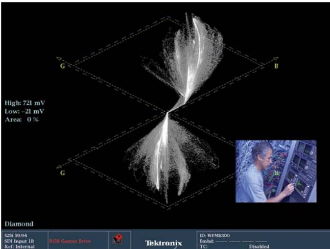
Figure 19. Live signal with blue balance error.
