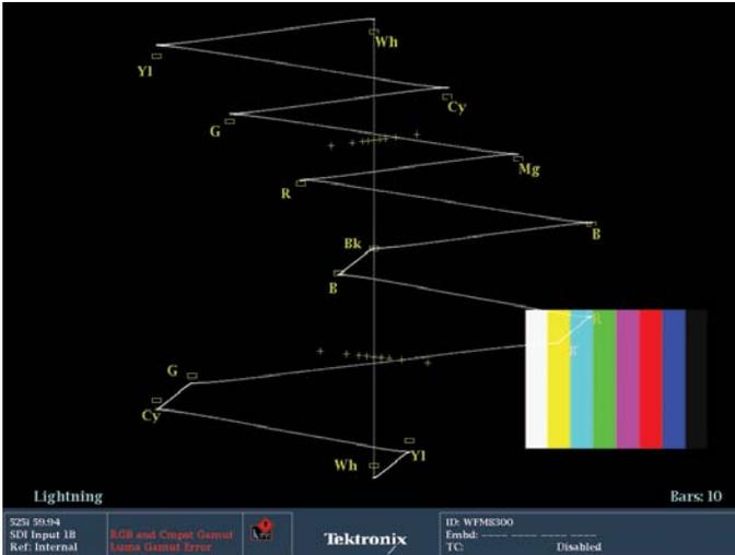
Figure 40. Luma gain error on Lightning display.
