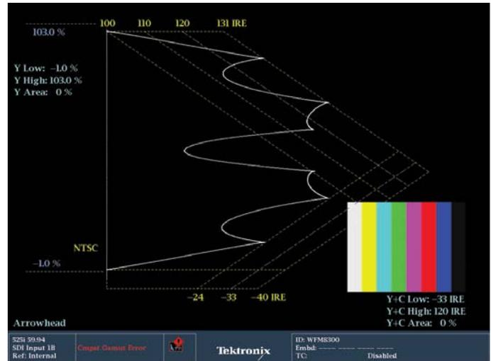
Figure 36. Arrowhead display with 100% Color Bars Signal.
