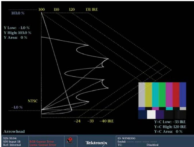
Figure 35. Arrowhead display showing SMPTE Color Bars.
