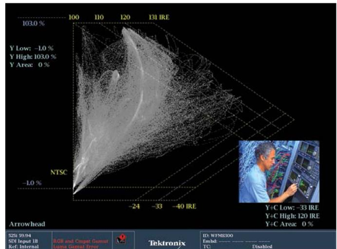
Figure 37. Live video signal monitored with the Arrowhead display showing clear indication of a composite gamut error.
