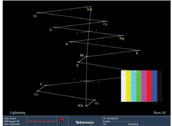
Figure 41. P'b gain error on Lightning display.
