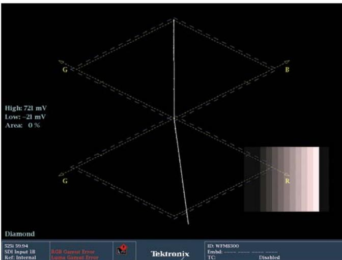
Figure 9. 10 step staircase with red imbalance.
