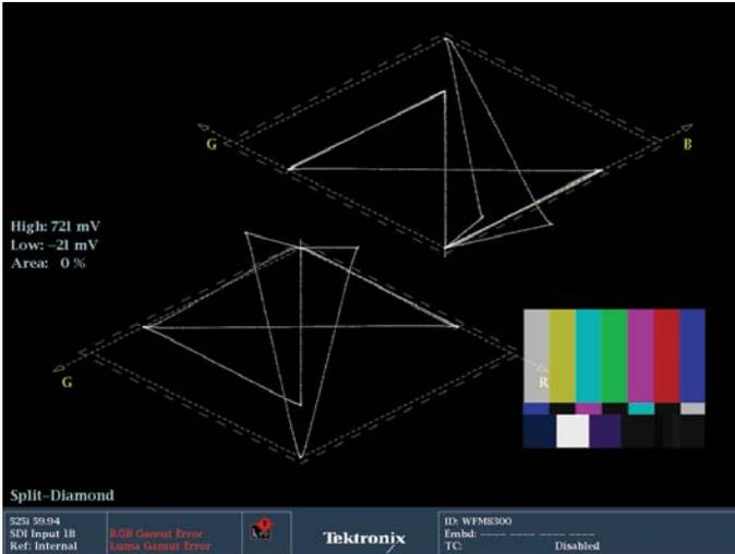
Figure 14. Split Diamond display using SMPTE Color Bars.
