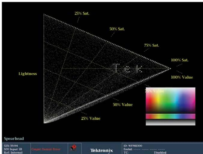
Figure 26. "Rainbow" test pattern on the Spearhead Display.
