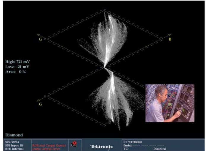
Figure 18. Live signal with red balance error.
