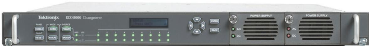
The ECO8000 electronic changeover unit works with a primary + backup pair of SPG9000 units to serve as a highly-reliable redundant system. It utilizes electronic fast switches for near glitch-less sync source switching, minimizing disruption in operation. Dual hot-swappable power supplies ensure continuous availability of reference signals, and signals are passed even when the unit is powered off.
