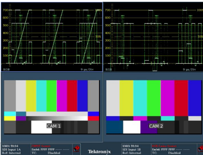
Two-channel simultaneous monitoring of waveform and picture input, ideal for monitoring multiple camera inputs.
