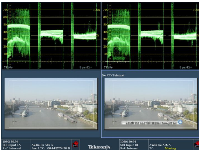
Simultaneous Input mode comparing incoming and outgoing signals
