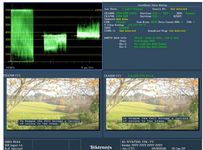
Simultaneous decode of CEA708 and CEA608 captions within multiple picture displays
