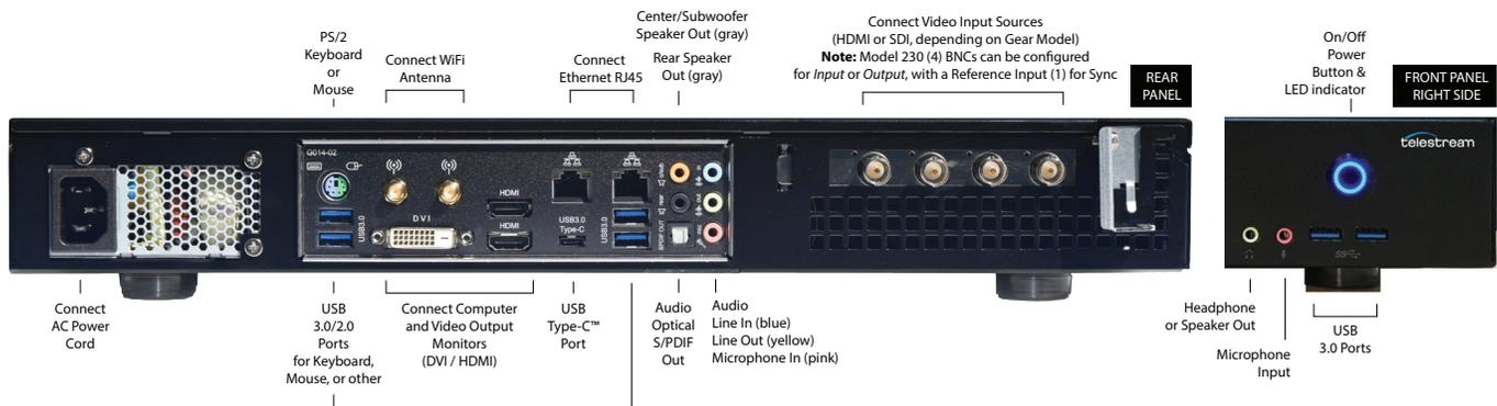
3. **Connect your computer monitor** to either the HDMI or DVI monitor output ports on the rear panel.
