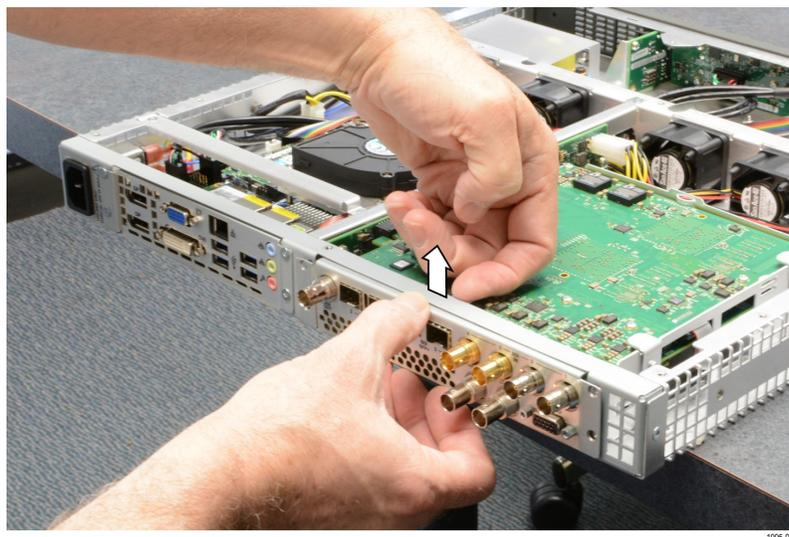
**Figure 27: Install the rear plate panel**
