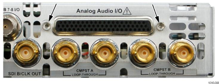
Figure 15: Audio connector retainer posts
