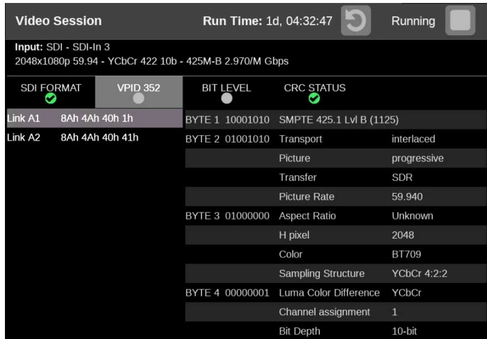
Figure 134: Video Session application — VPID-0352 tab display for 3G-SDI Level B signal
