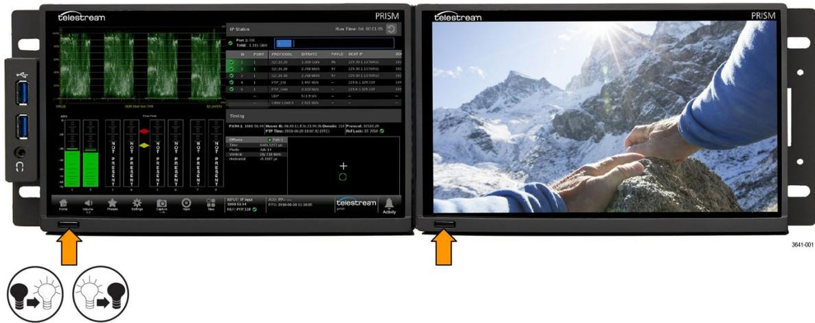
Figure 8: Extended display mode configuration with power buttons marked
