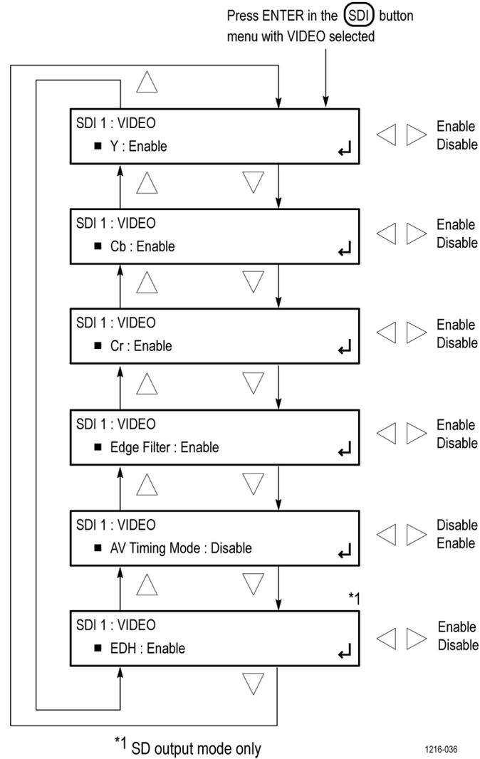
Figure 94: SDI VIDEO submenu diagram
