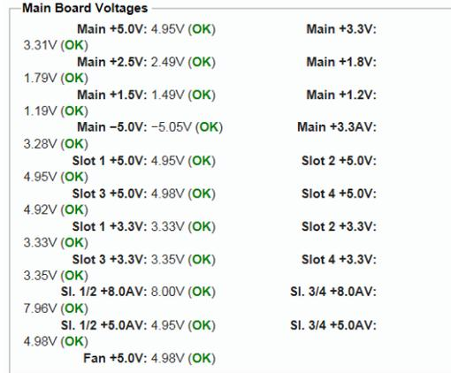
**Figure 48: Main Board Voltages diagnostic readouts**
