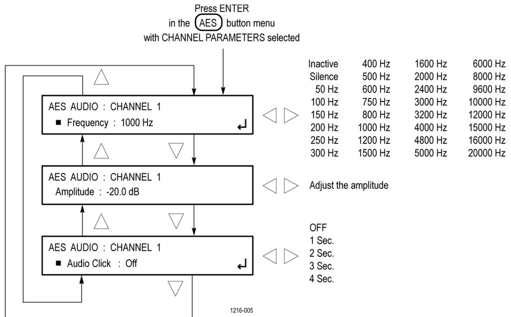
Figure 62: AES AUDIO CHANNEL submenu diagram (Option AG only)
