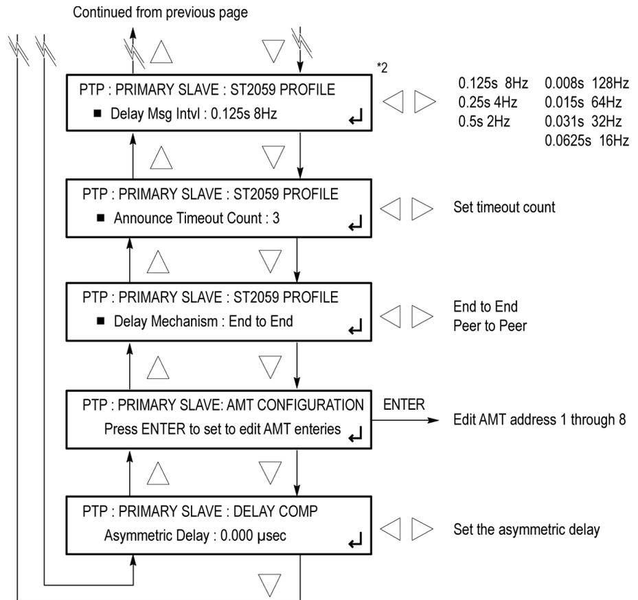
Figure 126: PTP primary slave menu diagram – part 2
