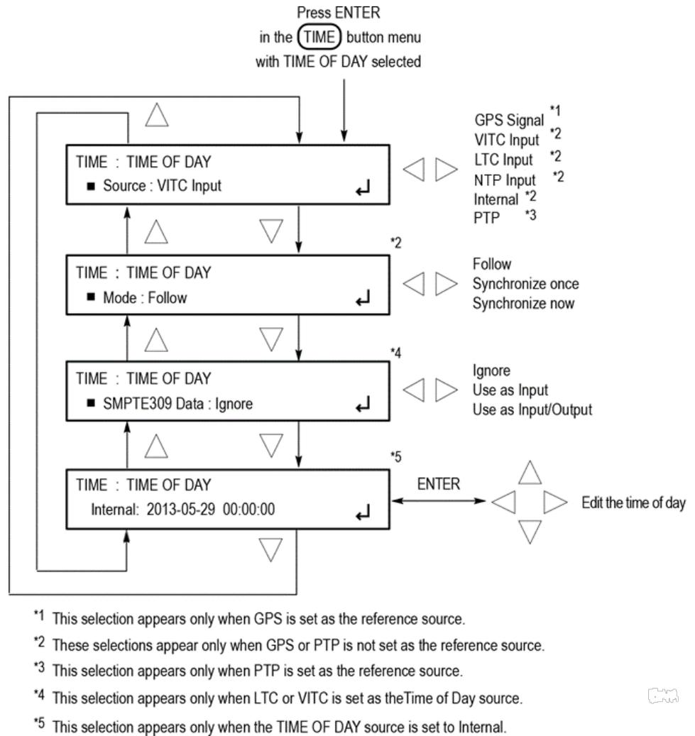
**Figure 118: TIME OF DAY submenu diagram**
