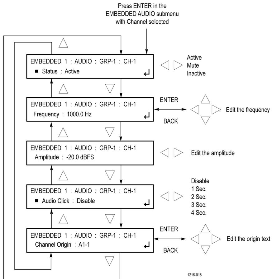
Figure 75: EMBEDDED CHANNEL submenu diagram
