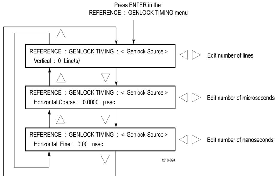
**Figure 82: GENLOCK TIMING submenu diagram**
