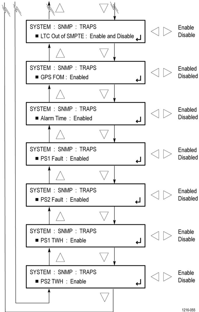
Figure 107: SNMP TRAPS submenu diagram – part 2
