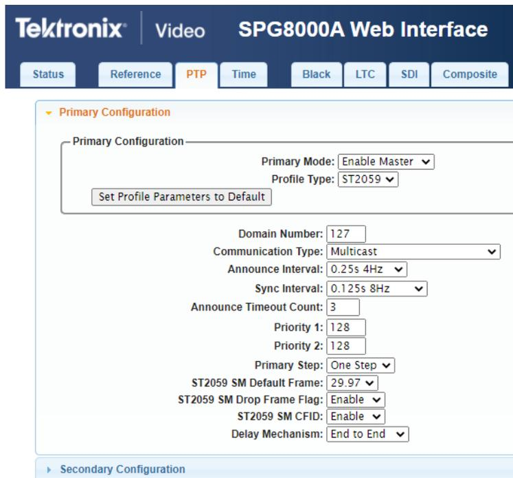
Figure 57: PTP Primary Master Configuration
