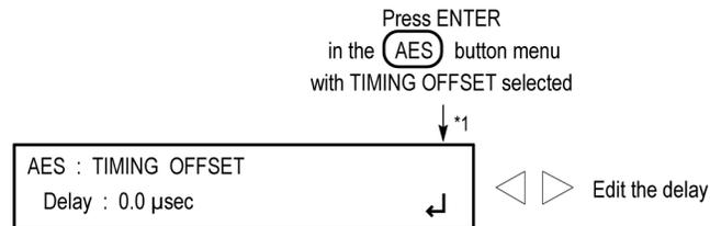
\*1 To adjust the offset, the AUDIO-VIDEO SYNC setting must be set to one of the frame reset signals.
