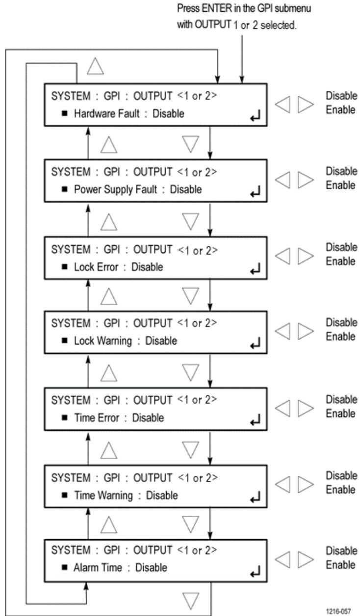
**Figure 109: GPI OUTPUT <1 or 2> submenu diagram**
