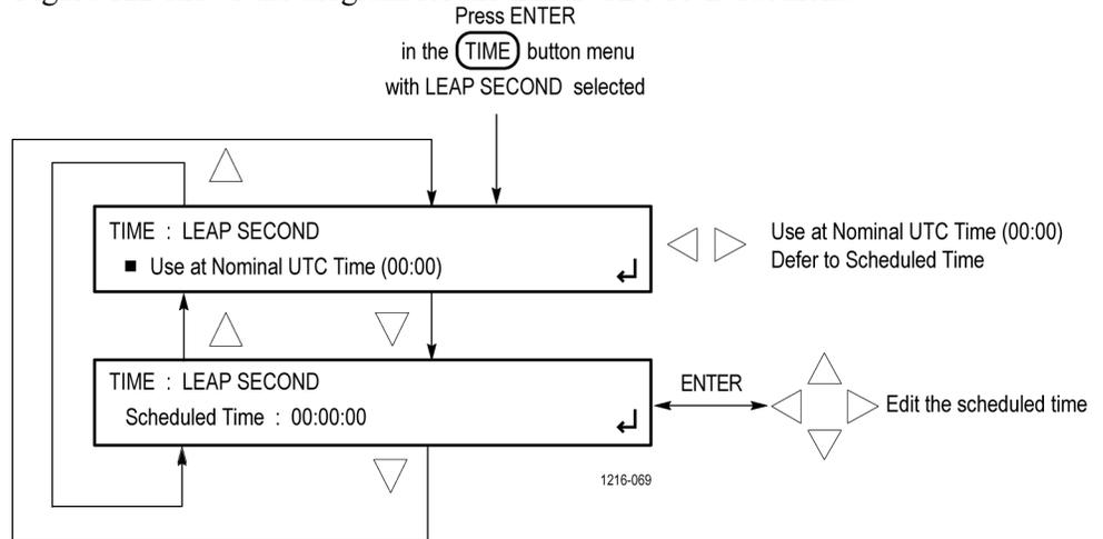
**Figure 122: LEAP SECOND submenu diagram**
