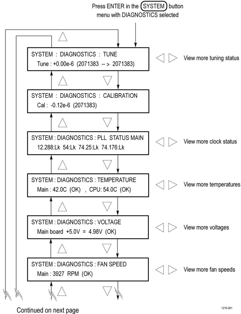
**Figure 114: DIAGNOSTICS submenu diagram – part 1**
