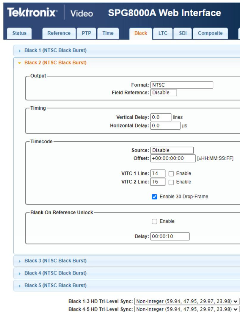
**Figure 9: Black menu with the Black 2 submenu expanded**
