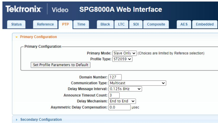
**Figure 58: PTP Primary Slave Configuration**
