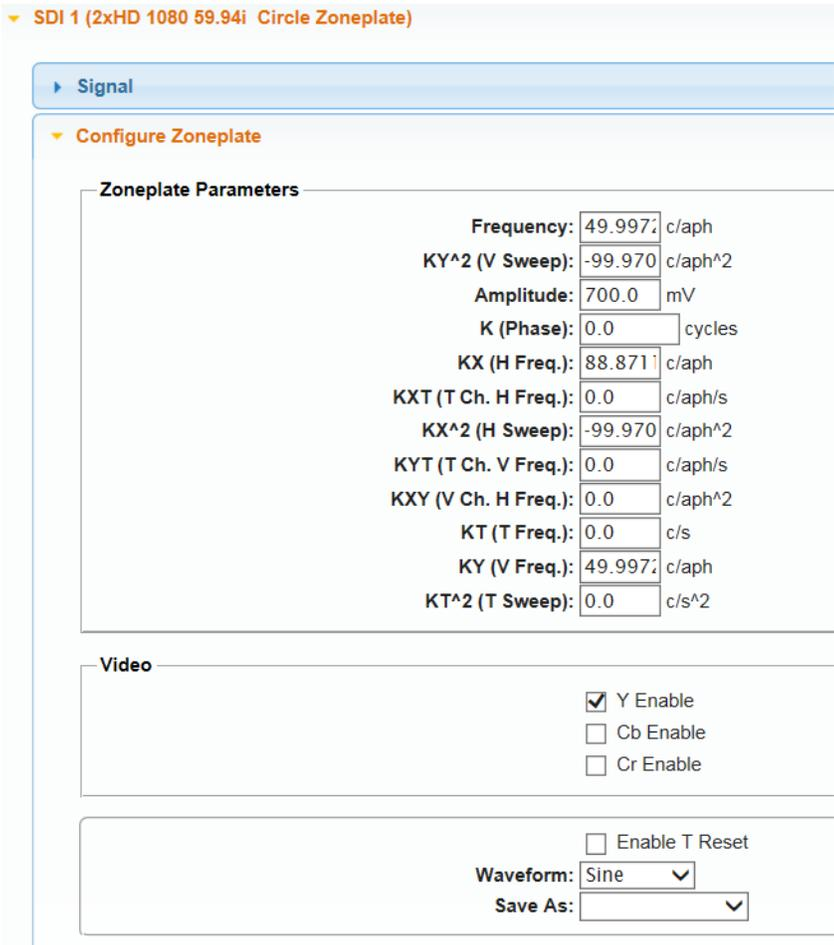
**Figure 17: Circle zone plate configuration parameters**
