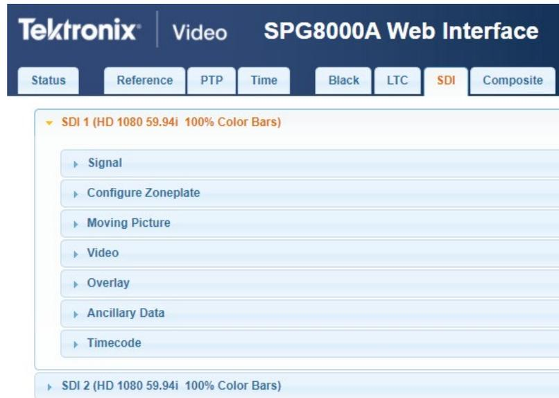
Figure 15: SDI menu with the SDI 1 submenu expanded
