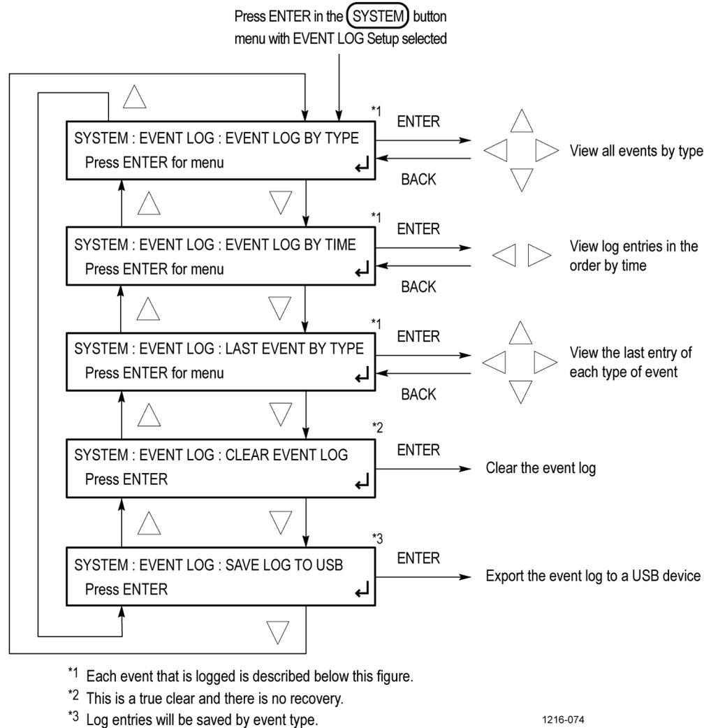
**Figure 113: EVENT LOG submenu diagram**
