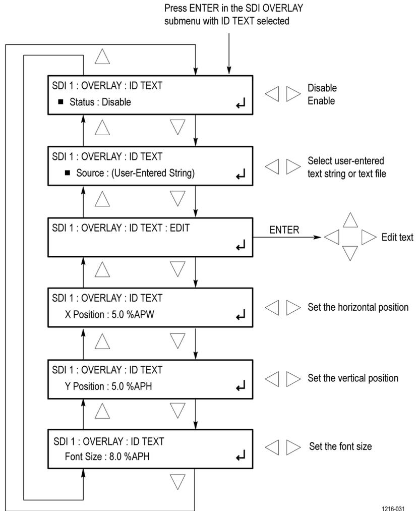
**Figure 89: SDI OVERLAY ID TEXT submenu**
