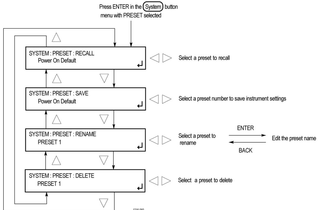
**Figure 102: PRESET submenu**
