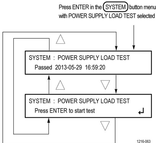
**Figure 116: POWER SUPPLY LOAD TEST submenu diagram**
