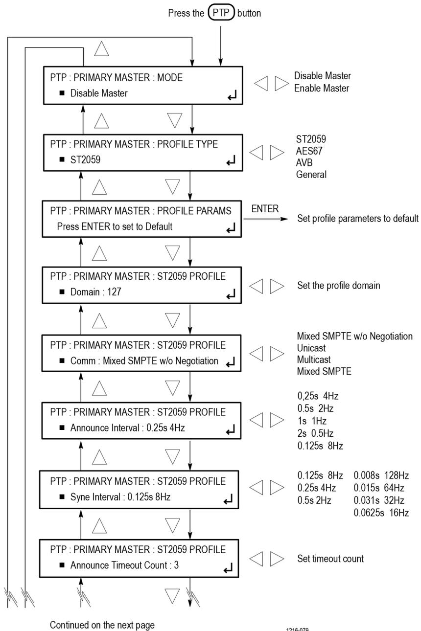
**Figure 123: PTP primary master menu diagram – part 1**
