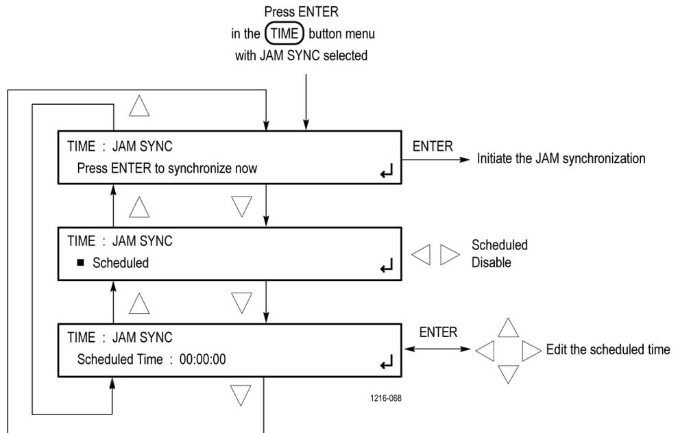
**Figure 121: JAM SYNC submenu diagram**
