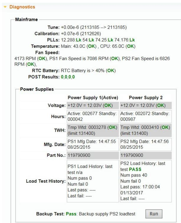
**Figure 46: Mainframe diagnostic readouts**
