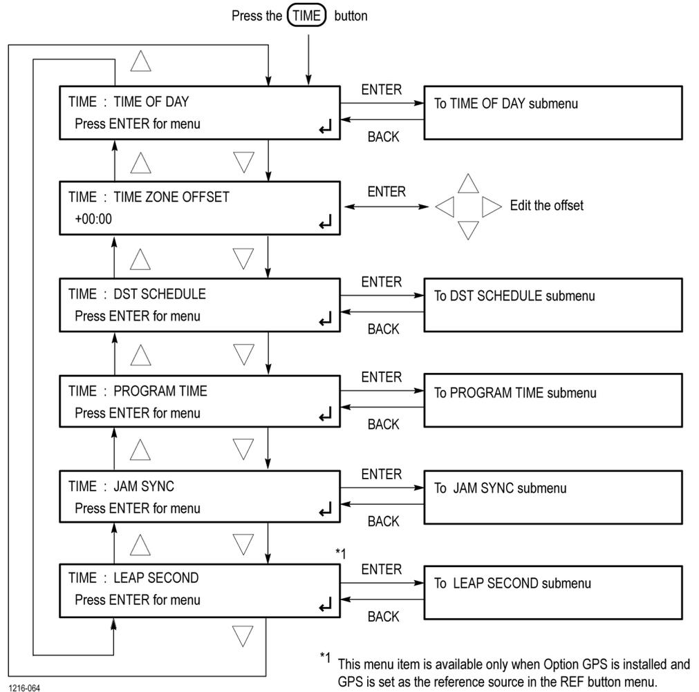
**Figure 117: TIME button menu diagram**
