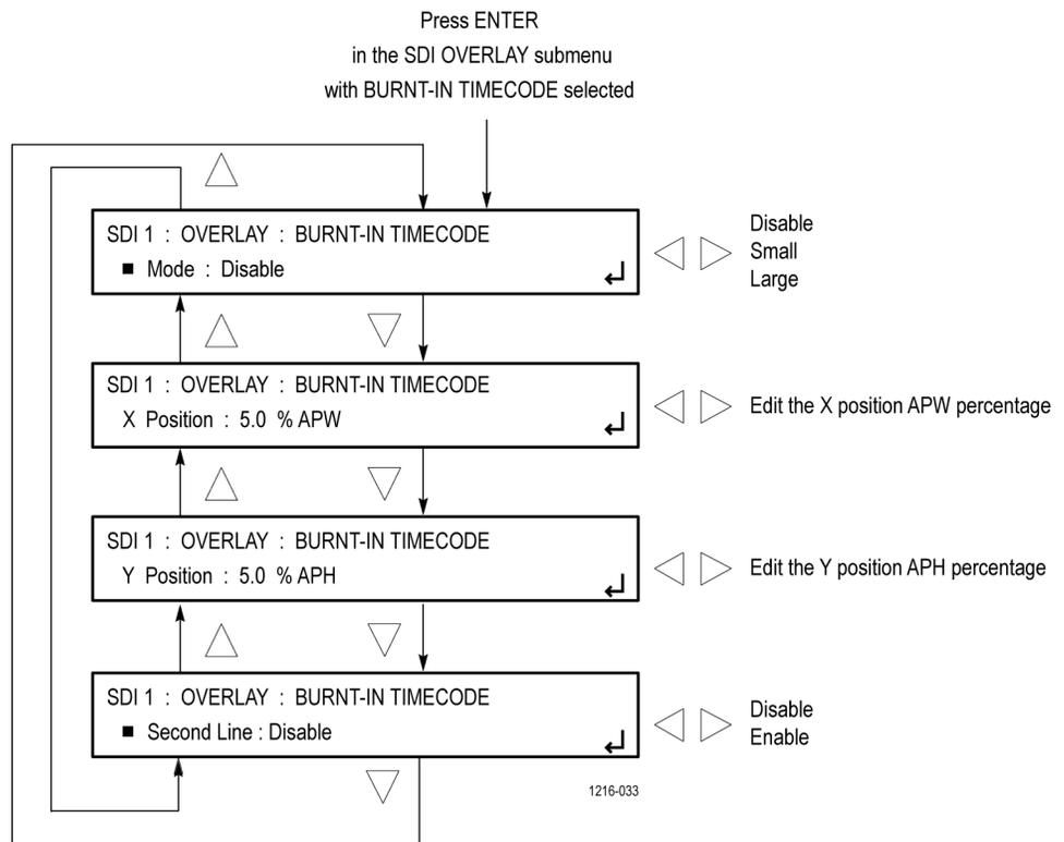
Figure 91: SDI OVERLAY BURNT-IN TIMECODE submenu
