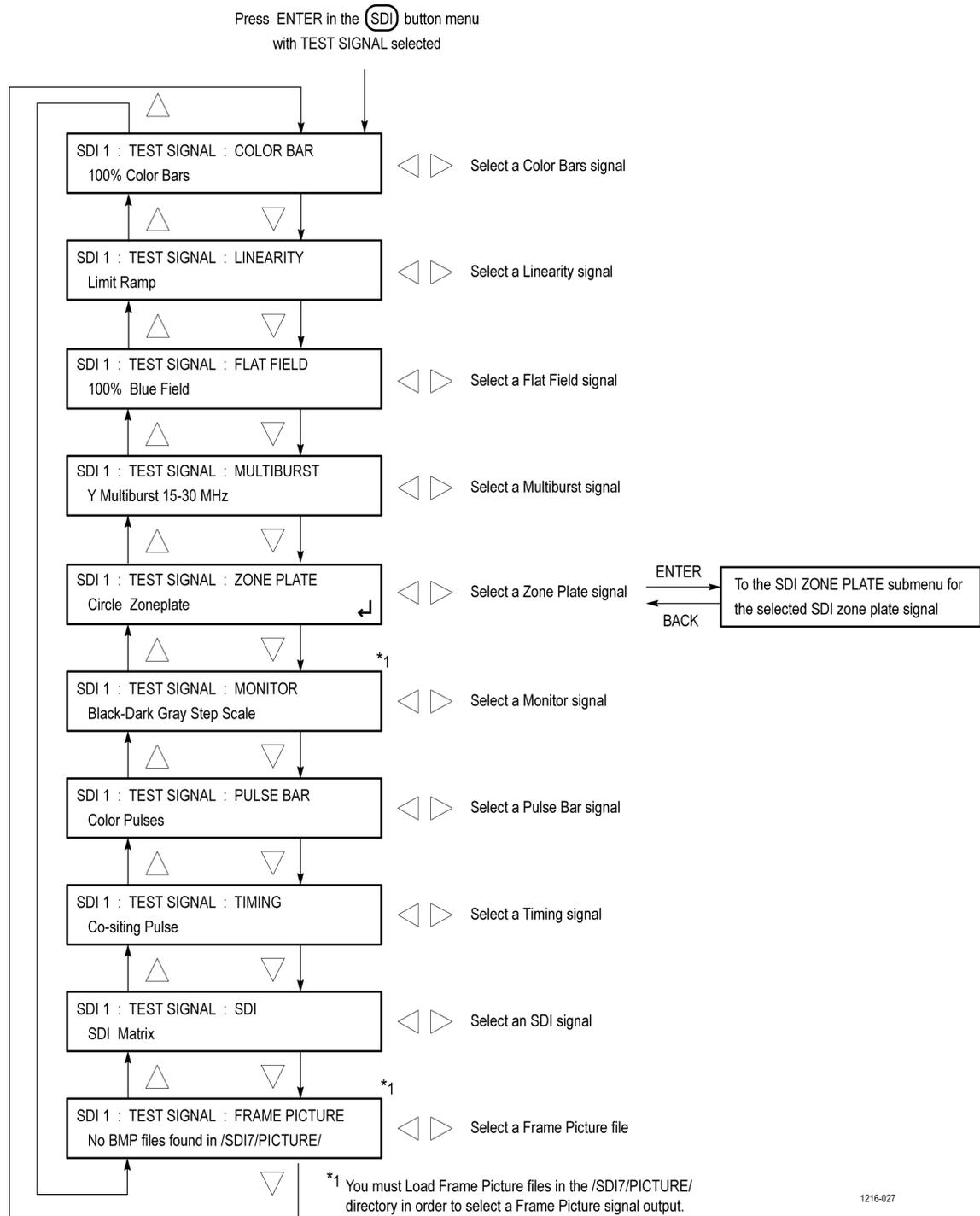
**Figure 85: SDI TEST SIGNAL submenu diagram**
