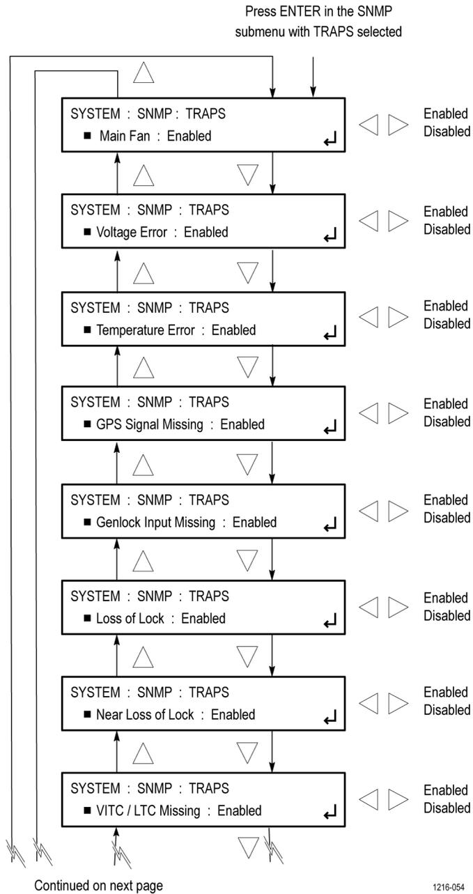
Figure 106: SNMP TRAPS submenu diagram – part 1
