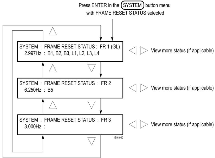
Figure 112: FRAME RESET STATUS submenu diagram
