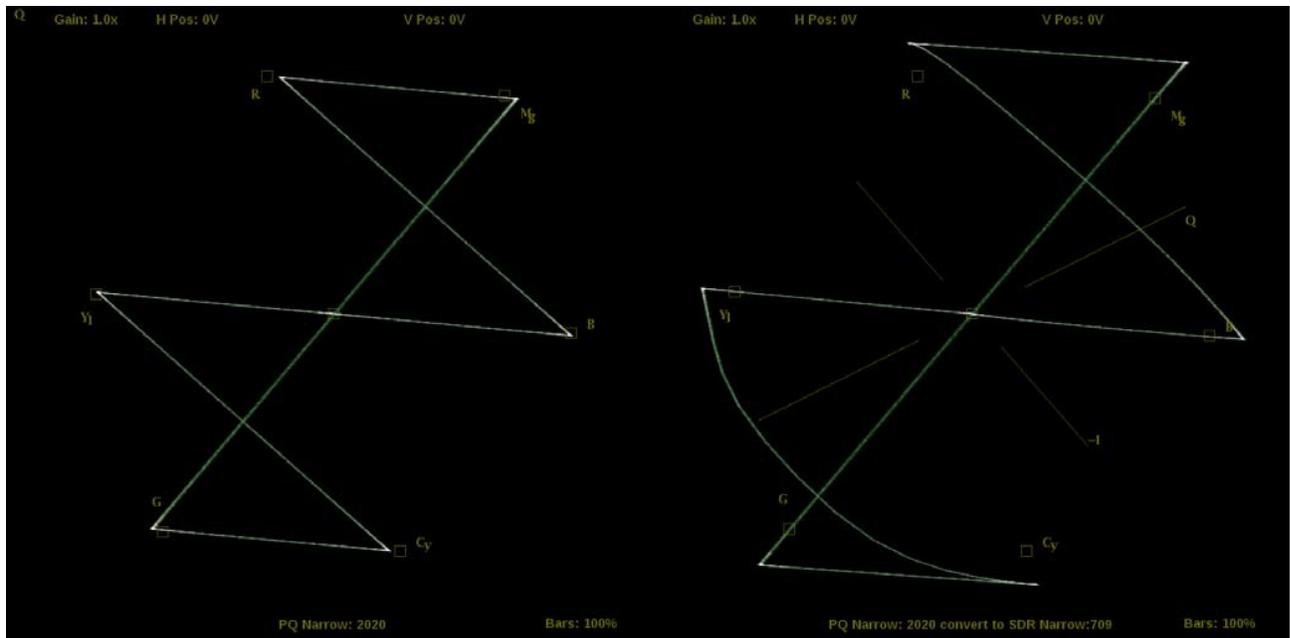
Figure 45: Vector display with (right) and without (left) Convert to Rec. 709 enabled, 100% color bar in PQ/BT.2020
