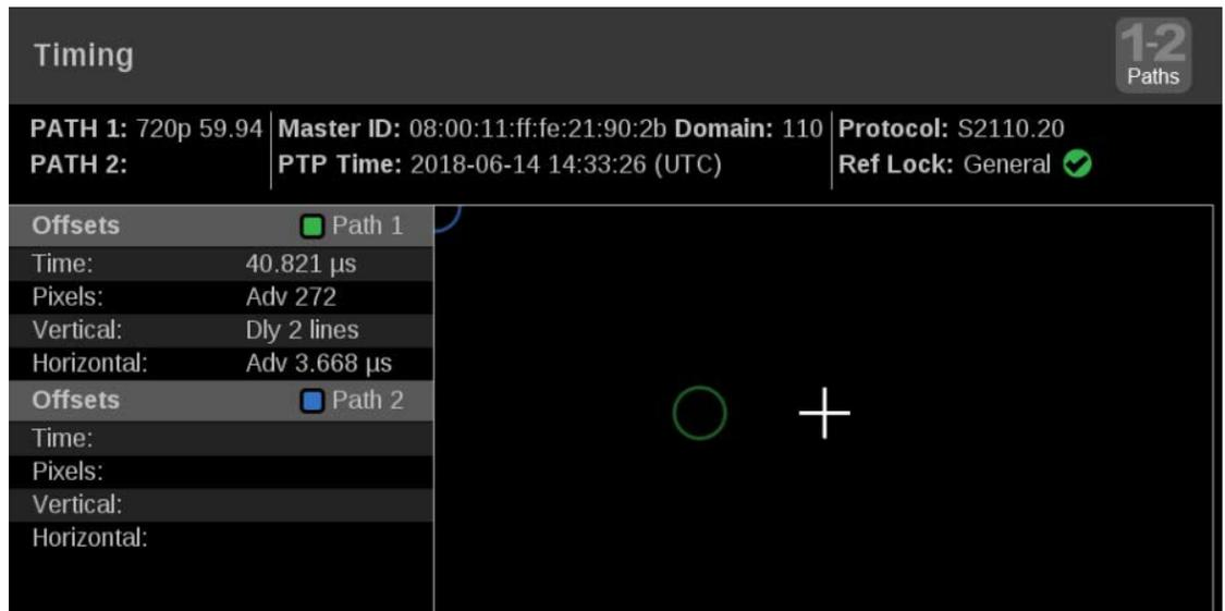
Figure 122: Timing application display for IP signals
