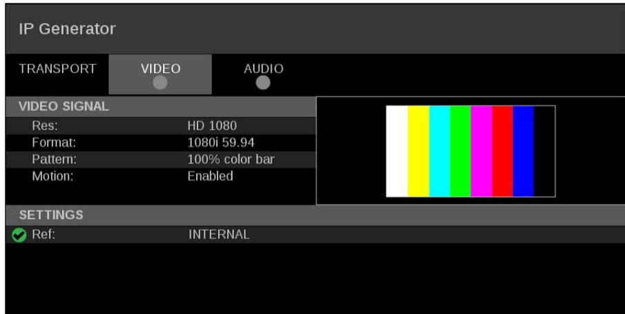
Figure 175: IP Generator application – VIDEO tab display
