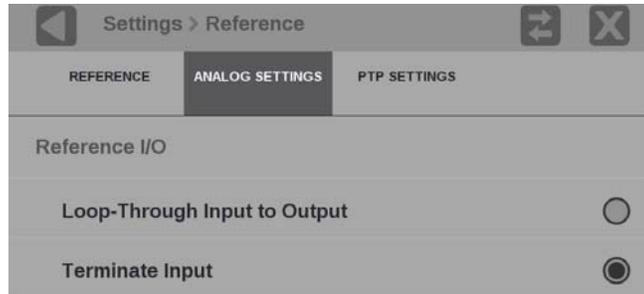
Figure 60: Analog reference settings configuration
