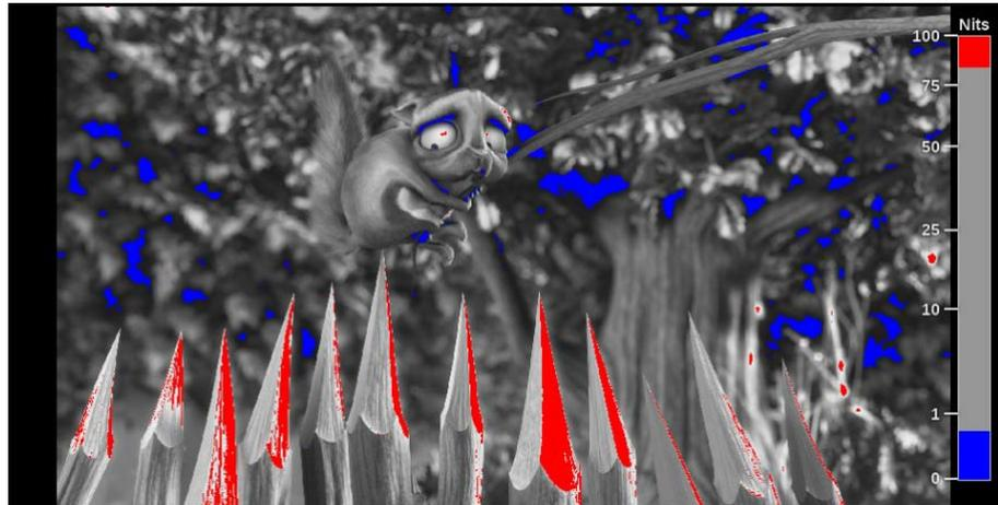
Figure 115: Luminance False Color display with Meter Overlay
