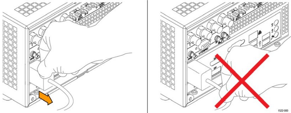
Figure 2: Disconnecting the power cord from the MPI2-10 monitor
