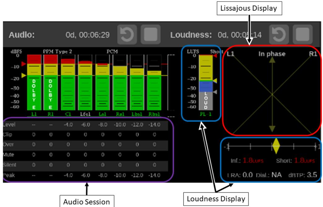
Figure 104: Elements of the Audio application display
