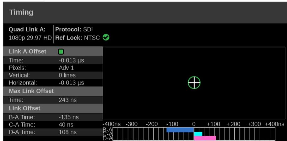
Figure 125: Timing application display for Quad Link SDI signals
