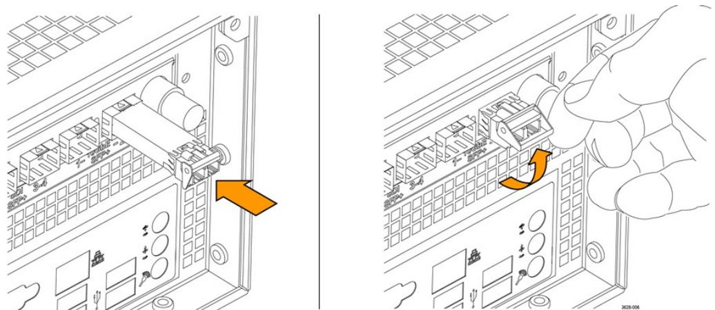
Figure 6: Installing and removing an optical SFP module on an MPI2-10 monitor
