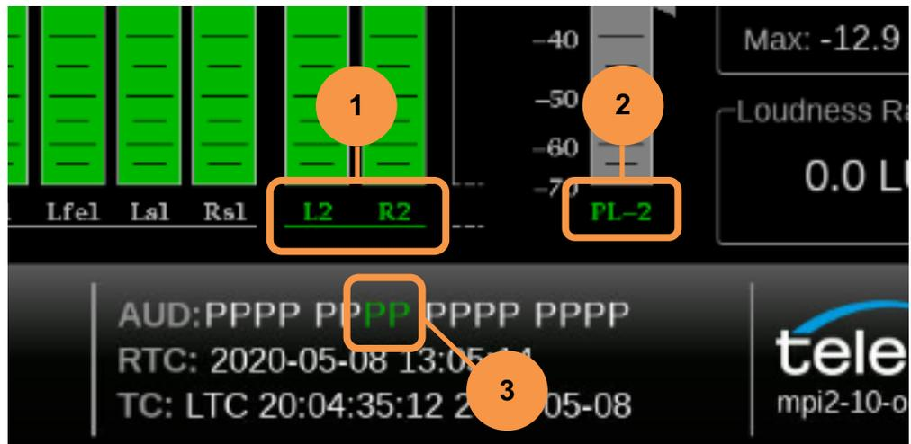
Figure 52: Program labels marked at the bottom of audio bars and in the status bar
