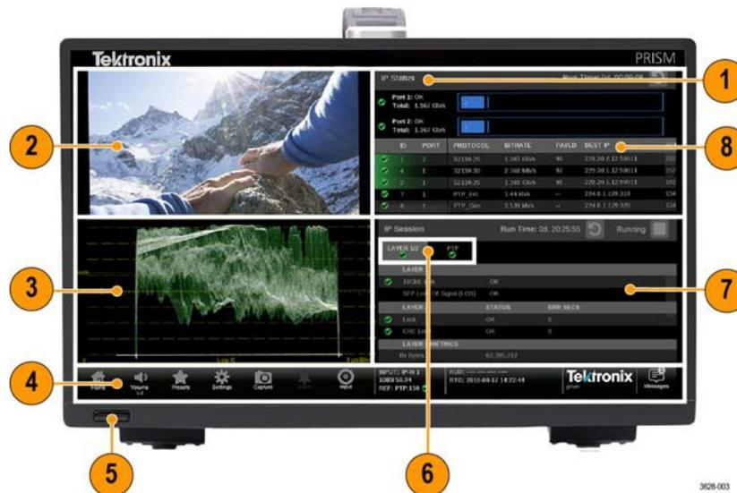
Figure 12: Elements of the display (MPI2-10 monitor shown)
