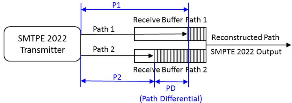
Figure 150: Seamless protection switching of SMPTE ST-2022-7 IP stream
