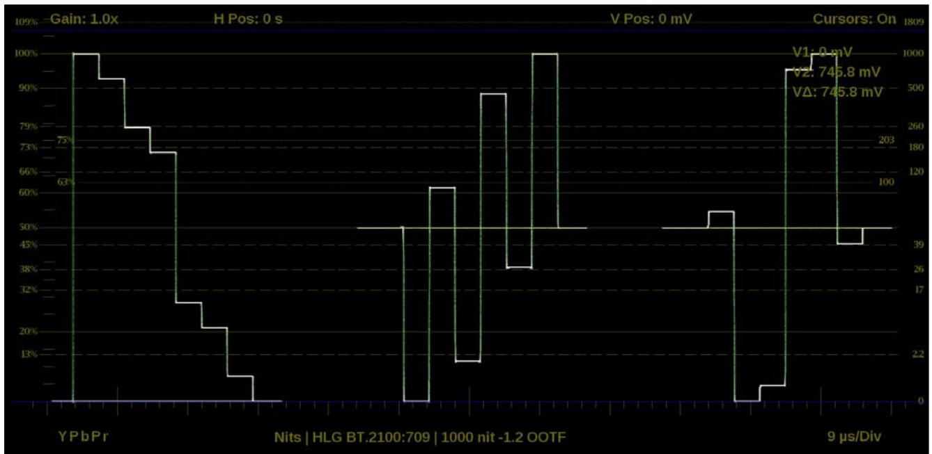
Figure 43: Waveform display with nits scale
