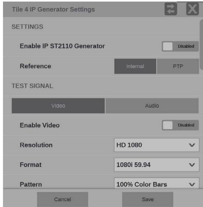
Figure 171: IP Generator application settings menu
