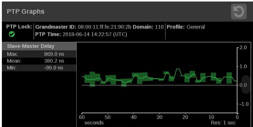
Figure 159: PTP Master-Slave Delay and Variation graphs
