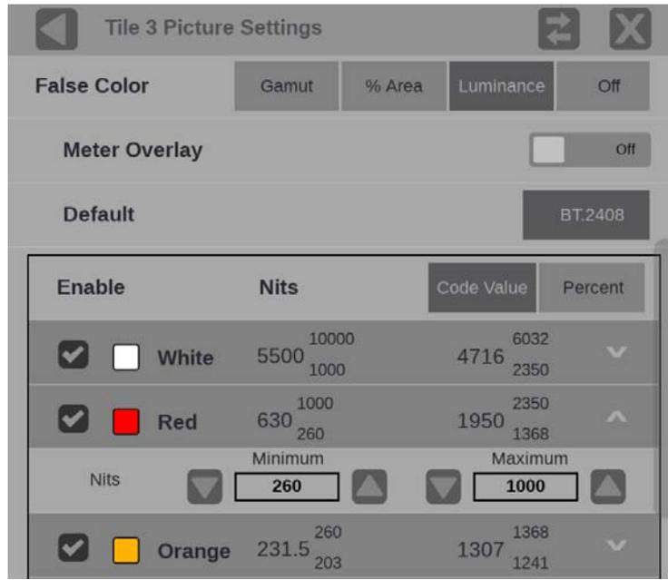
Figure 116: Picture settings with the Luminance False Color table
