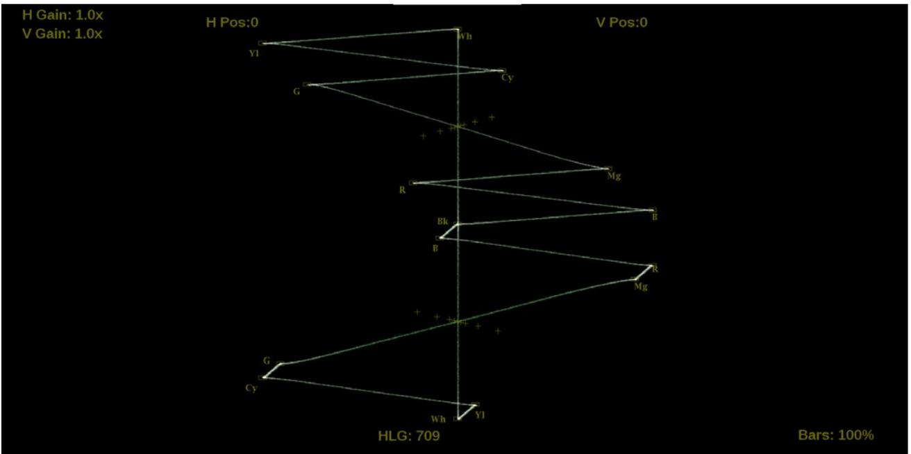
Figure 205: Lightning display application
