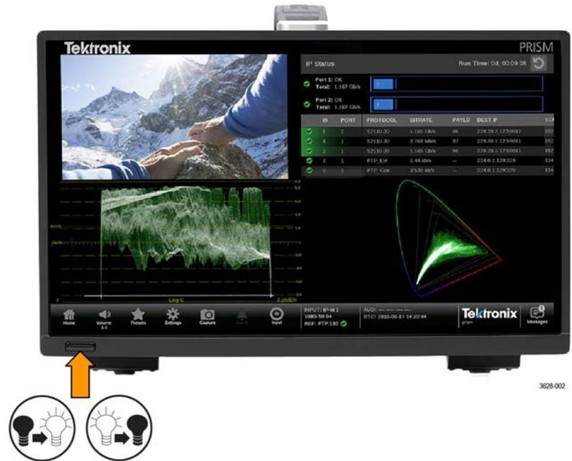
Figure 3: Front panel of the PRISM with the Power/Standby button marked
