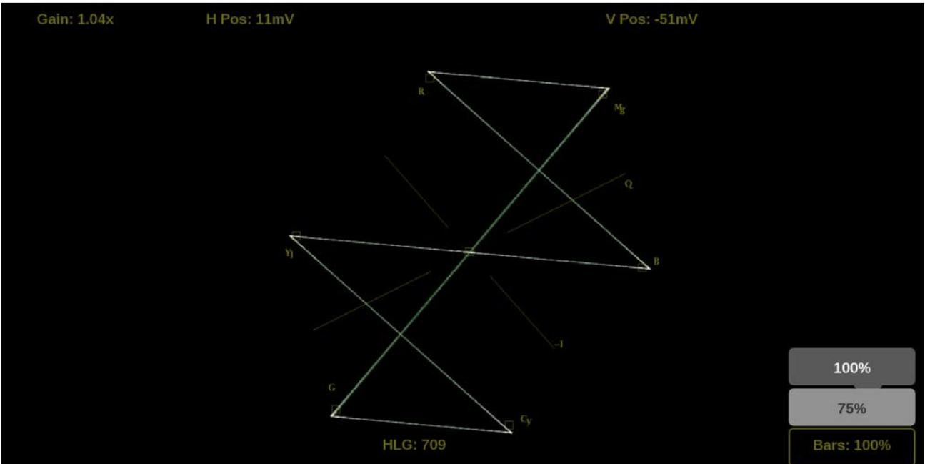
Figure 99: Vector on-screen tools – Bar Targets
