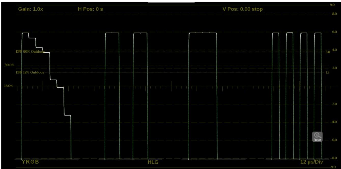
Figure 44: Stop Display with Stop scale
