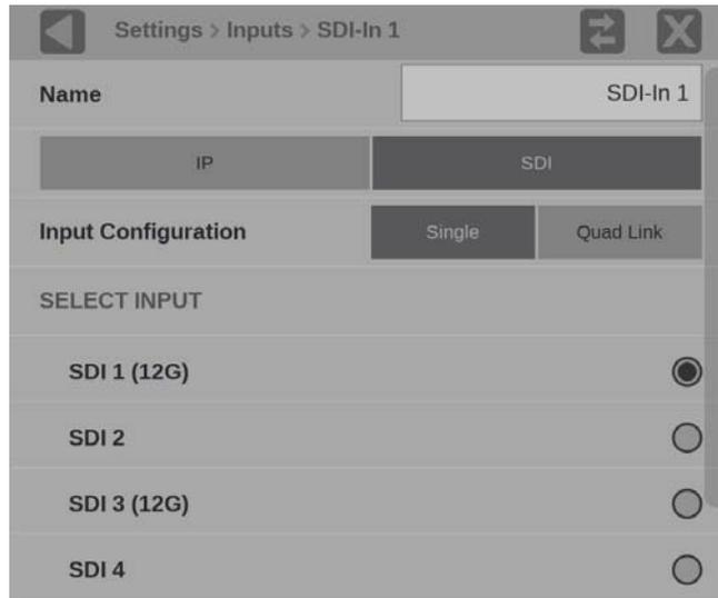
Figure 29: Single SDI signal configuration
