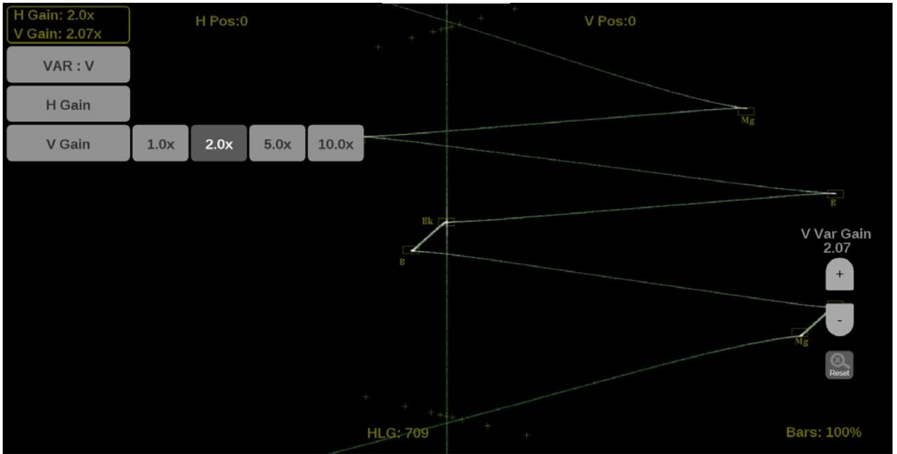
Figure 210: Lightning on-screen tools – vertical gain
