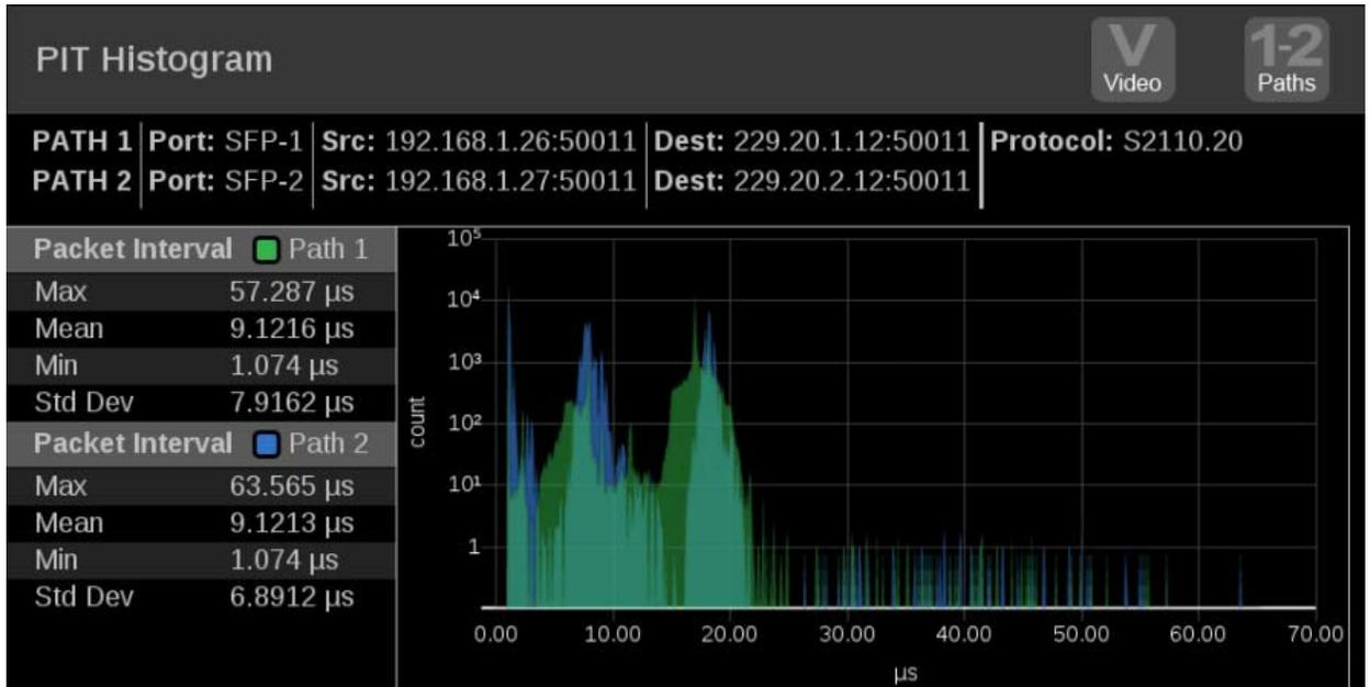
Figure 153: PIT Histogram application display
