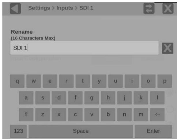
Figure 34: Renaming a signal input
