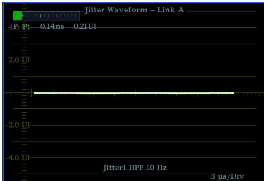
Figure 32: The Jitter display parameters as shown in a single tile when the instrument is in 4-tile mode
